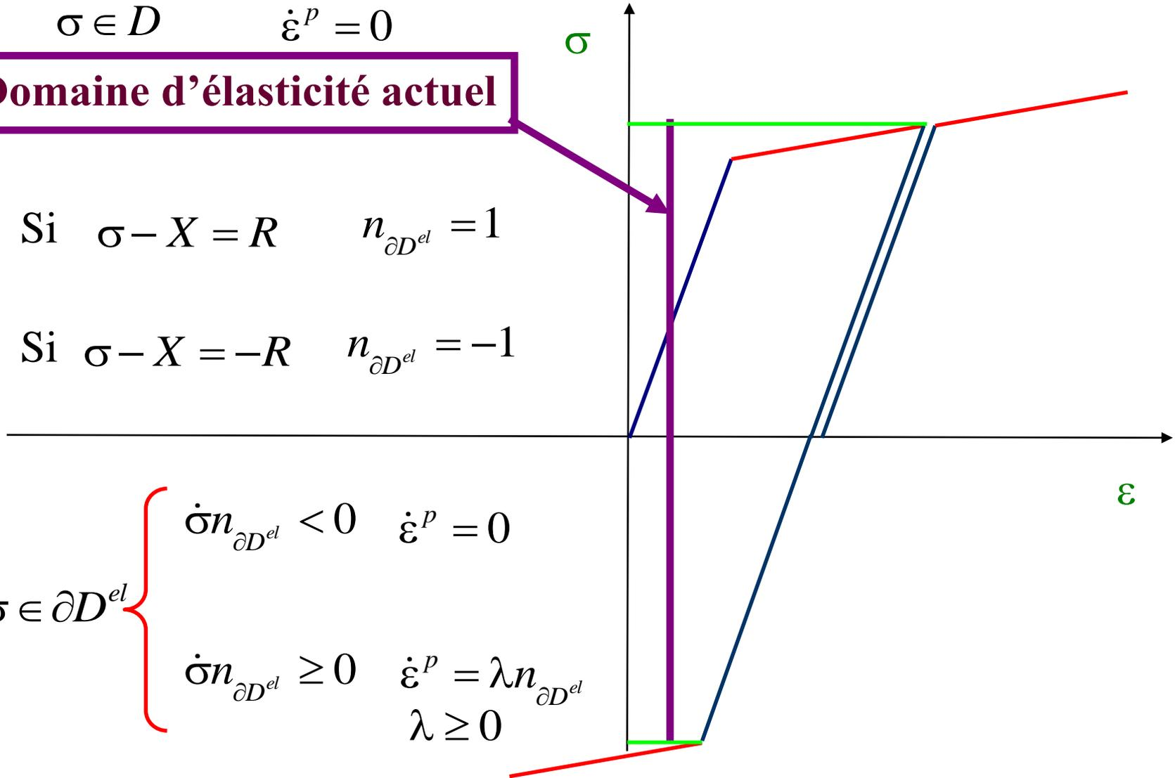
Si  $\sigma \in \partial D^{el}$   $\left\{ \begin{array}{l} \dot{\sigma} n_{\partial D^{el}} < 0 \quad \dot{\varepsilon}^p = 0 \\ \dot{\sigma} n_{\partial D^{el}} \geq 0 \quad \dot{\varepsilon}^p = \lambda n_{\partial D^{el}} \\ \lambda \geq 0 \end{array} \right.$
